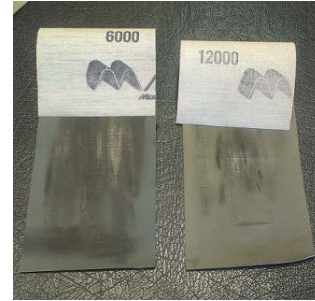
Fig. 3.2.2: Two different types of Abrasive sandpaper of Micro-Mesh Company used for polishing.
